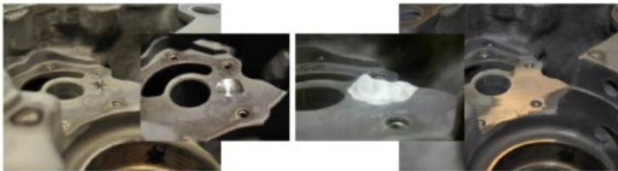
As-Received → Pre-Machined → Cold Sprayed → Finish Machined
