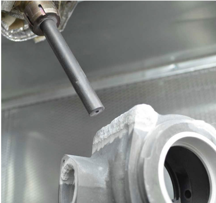
[1] Cold spray Repair, COC Aerospace, http://www.coc-aerospace.com/portfolio-item/case-study-1/
