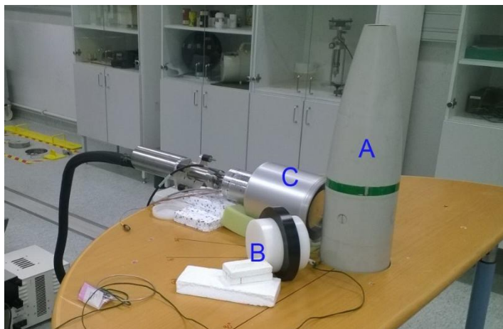
Figure 1. Measurement setup. The grenade shell filled with materials under scrutiny is in the middle (A) partially submerged into the table, the neutron source is inside the white plastic tube supported with black plastic ring (B), the detector system is housed inside a lead casing which is inside aluminium tube (C).
